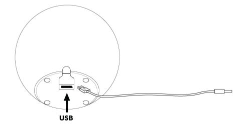
2. Connect the USB cable from the drive to the computer.
